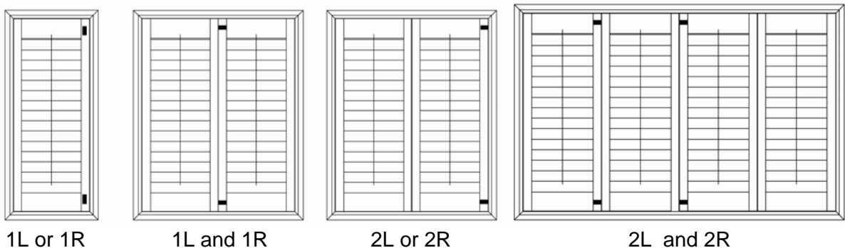
Panel Configurations with Magnet Positions in Black
